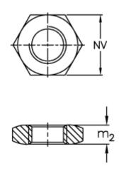
$\begin{array}{ll} m2 &= 9.0\\ Nominal size &= M18\\ NV &= 27.00\\ Thread pitch &= 1.50\\ Weight (g) &= 28.0 \end{array}$
